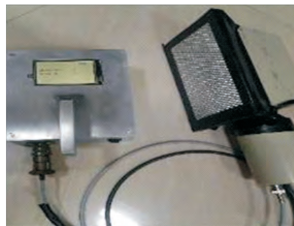
Fig. 10: Prototype of indigenously developed alpha and beta contamination monitor
