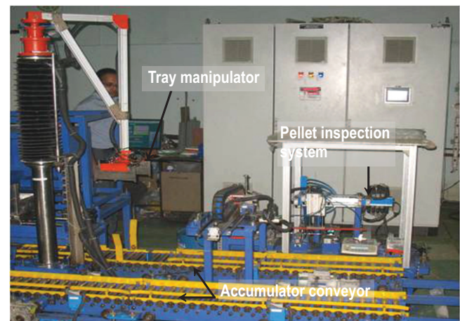
Tray Manipulator and Pellet Inspection Facility
