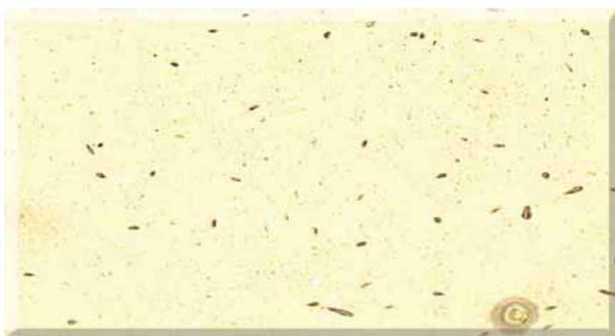
Fig. 5: Fission tracks per field ( 1.91 \times 10^{-3} \text{ cm}^2 ) observed under 400X magnification
