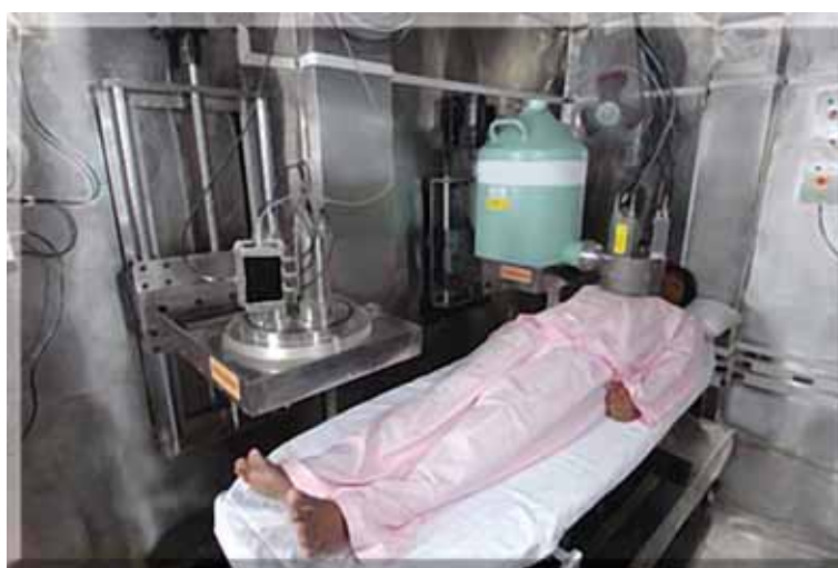
Fig. 2: A person is being monitored for lung contamination using LOAX HPGe detector.
