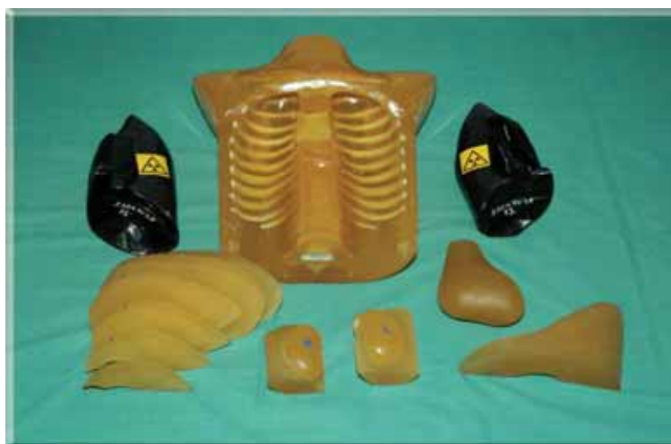
Fig. 10: JAERI phantom with its internal parts
