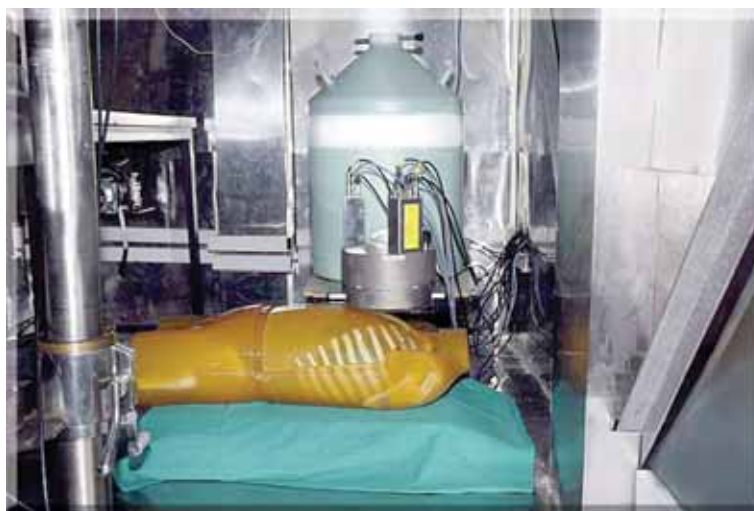
Fig. 1: LOAX HPGe detector and JAERI phantom in counting position inside the steel room
