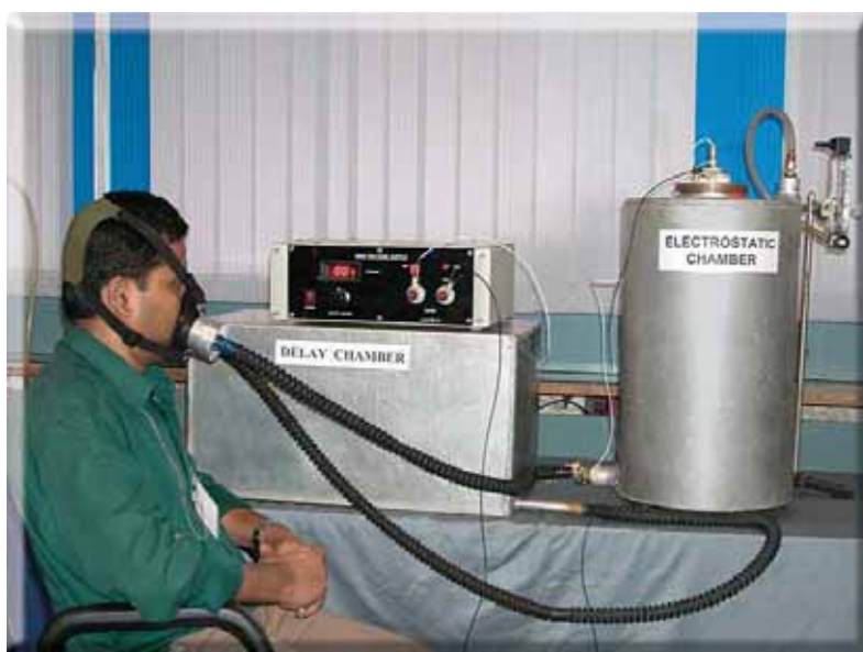
Fig. 6: A TIBM instrument is being used for monitoring of a worker due to possible contamination from thorium
