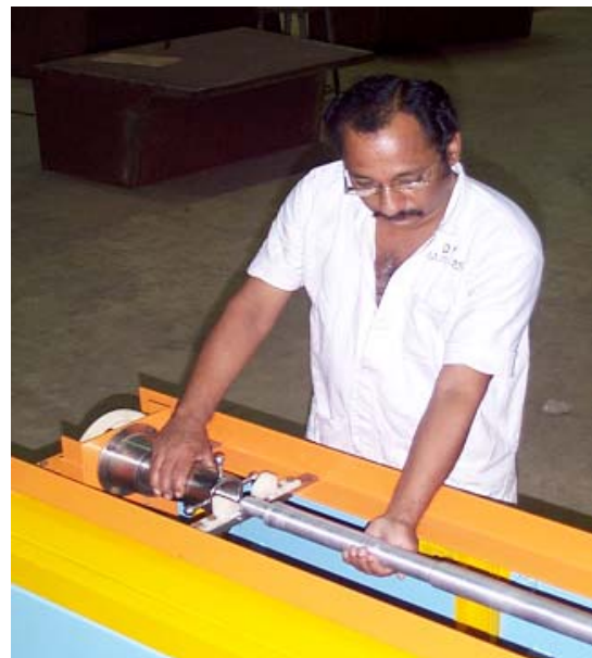
Fig. 8 Loading procedure of the fuel bundle
