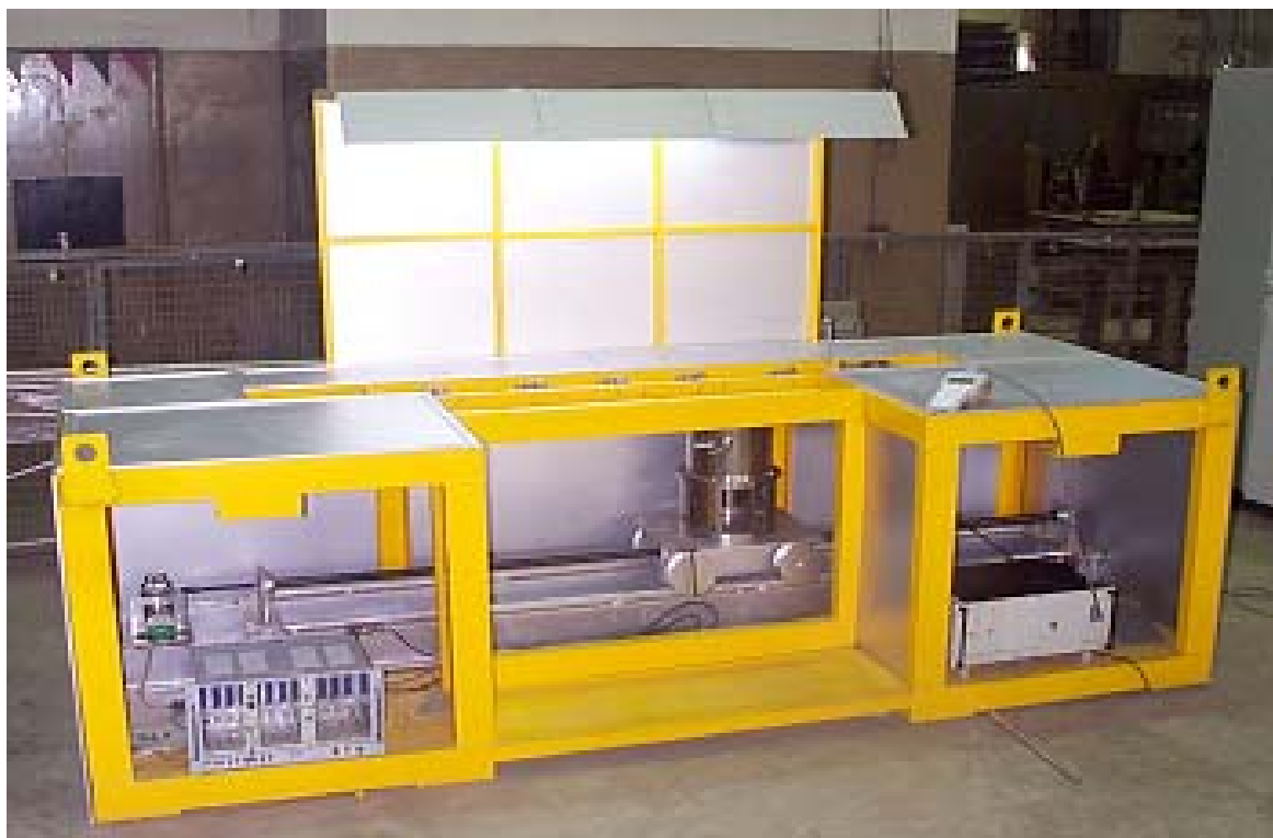
Fig. 6 Prototype of fuel pin scanner
