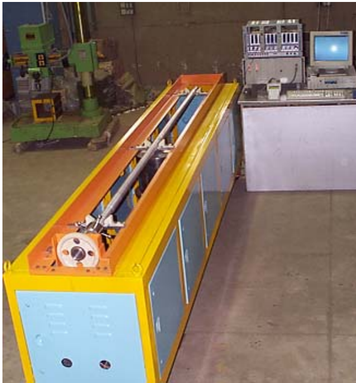
Fig. 7 Test set-up for prototype fuel bundle scanner
