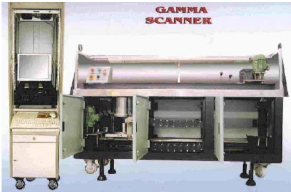
Fig. 9 Fuel pin scanner
