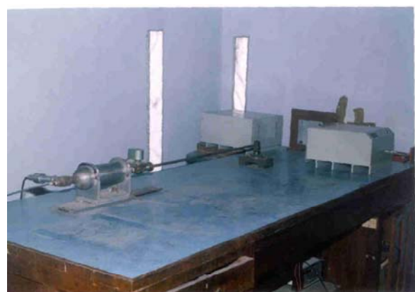
Fig. 5: Testing of Laser Velocity Meter with table-top gas gun
