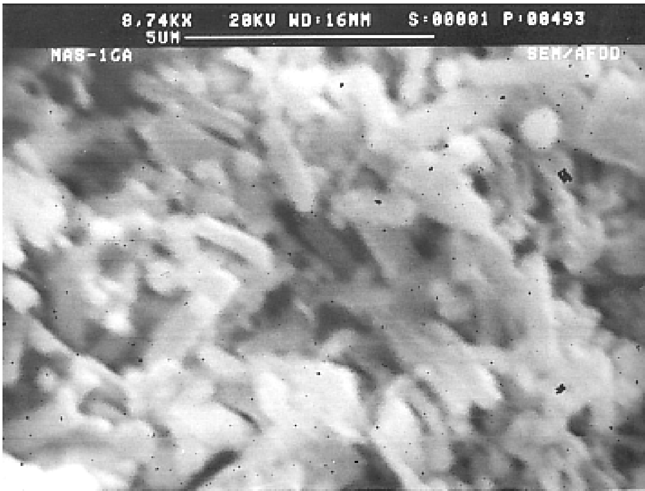
Fig.2 Microstructure of machinable quality MAS glass-ceramic having interlocking plate-like structure
