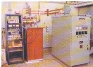
Fig. 1 Experimental set-up to measure critical current of superconducting wires.
