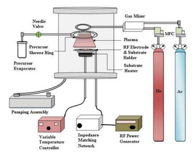
Figure: Simplified schematic of the RF-PECVD system
