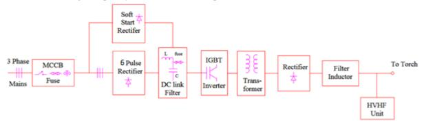
Conceptual block diagram of typical DC plasma power source
