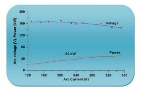
Typical V-I characteristics for the plasma torch is shown in figure above. The arc voltage remains nearly constant over a range of currents. A slight drop in the voltage is observed at higher currents. Increase in power with increase in current is slightly non-linear. For operation around 50 kW the torch operates near current 350 A and voltage 156 V.
