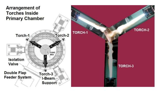
Three plasma torches discharging inside coke bed of primary chamber
