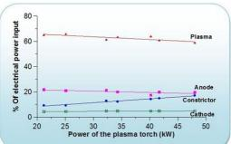
Power delivered into the plasma by the power supply is partly dissipated in heating the anode, constrictor and the cathode system. Rest of the delivered power goes into the plasma. As seen in figure, less than 5 % of the total input electrical power is dissipated by the cathode. The torch efficiency is nearly 65% around 20 kW and around 60% at 50 kW. In transferred arc mode, only loss is due to the cathode and efficiency goes above 95%.
