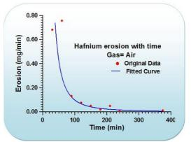
As shown above extremely low electrode loss due to erosion is observed for the cathodes. For new electrodes, the loss is relatively high at the start but decreases fast with time and stays at that extremely low level. The electrode loss reduces with increase in current.
