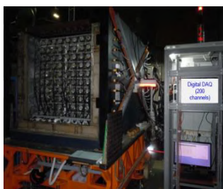
ISMRAN detector with passive shielding inside Dhruva reactor hall
