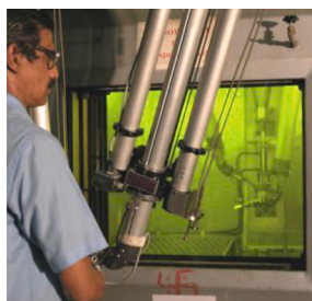
Tray Rod Facility (TRF) window and Master-Slave manipulator
