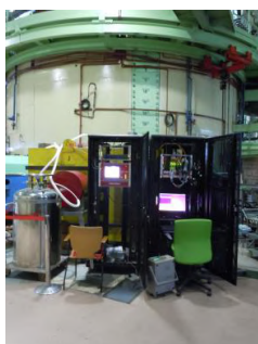
Digitizer based data acquisition system and control panel
