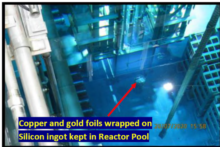
Neutron flux characterization and Si irradiation in out of core region of Apsara-U
