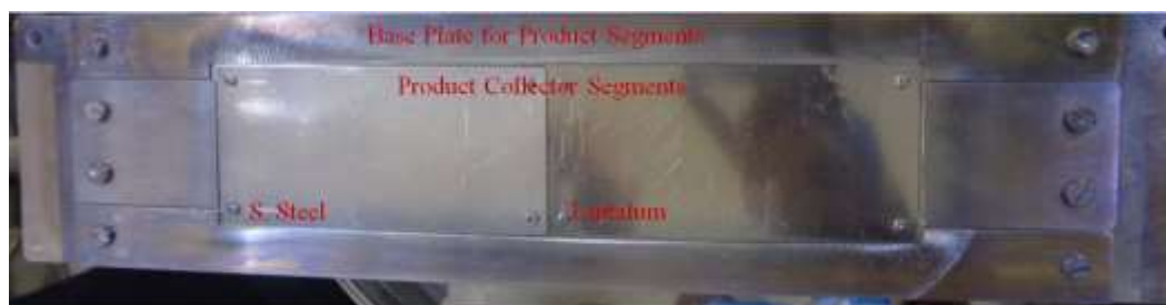
Fig 1: Product collector segments made of stainless steel and tantalum mounted on base plate
