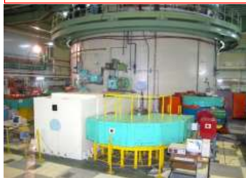
Fig.1. Neutron Powder Diffractometer (PD-III) developed by UGC-DAE CSR, Mumbai Centre. (above) Schematic of beamline and (below) actual instrument
