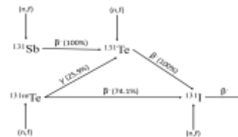
Fig. 1(b): Production of ^{131}\text{I} from fission
