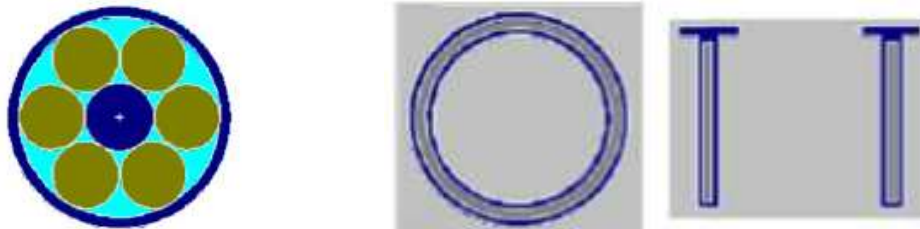
Fig. 1: 6 pellet design (6mm dia pellet) Fig. 2: annular arrangement of 1 mm dia pellet
