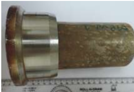
Fig.1.AA5052 tube OD 70mm x 2mm thick to SS304 end sheet in expansion mode. Joint after 500 thermal cycles (300K and 373K)
