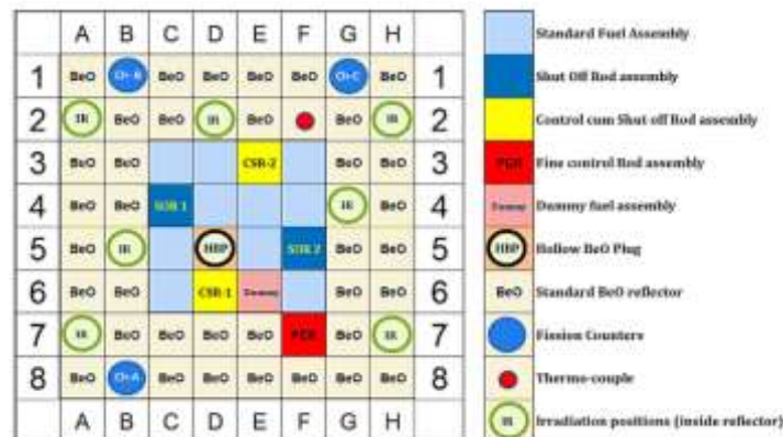
Fig. 1: Irradiation positions of Apsara-U along with the core configuration
