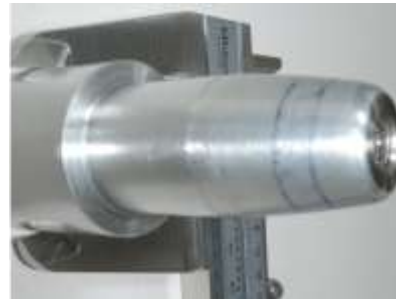
Fig.2.AA5052 tube (OD 22mm x 2mm thick) to SS304 end plug in compression mode, HL rate < 1.5 \times 10^{-10} mbar.l/sec
