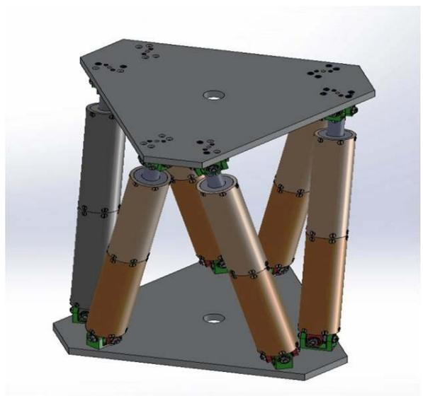
Fig.4: Isometric 3 dimensional view of miniature hexapod
