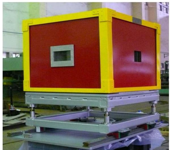
Fig.5: Collimator assembly with stand assembly
