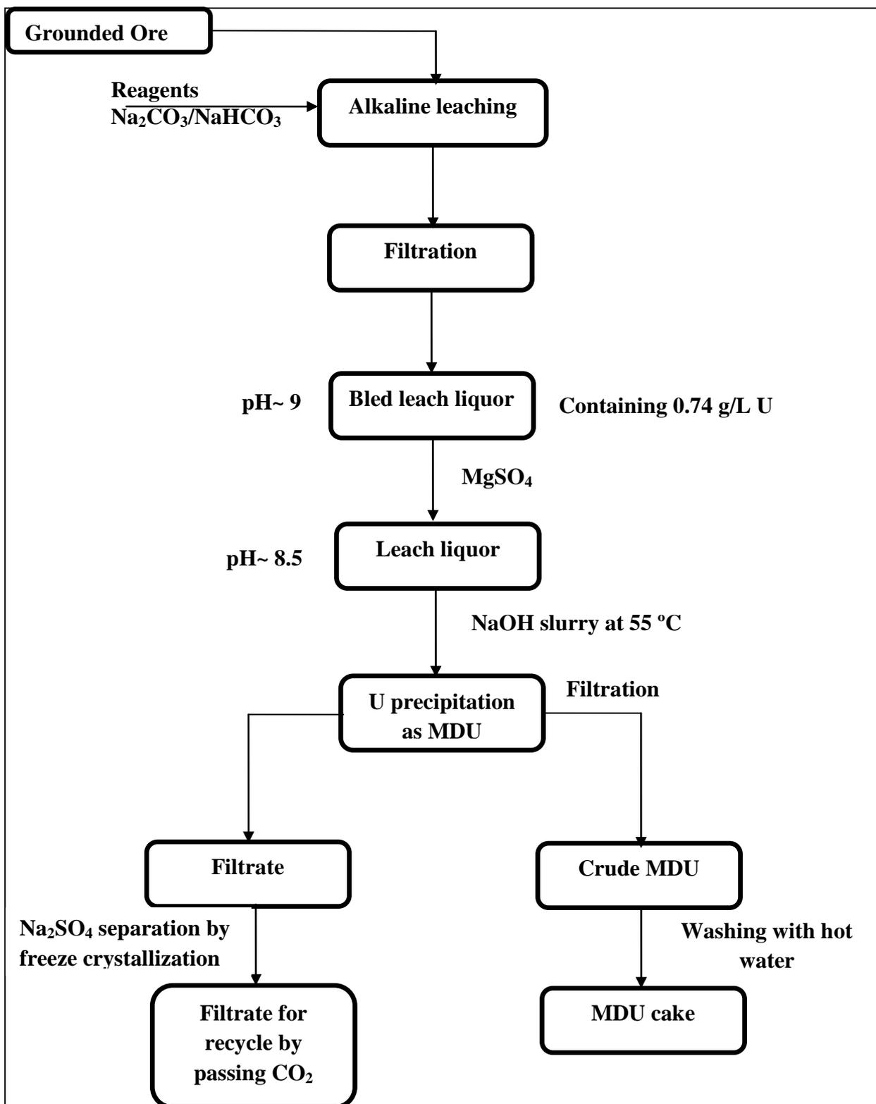
Figure 1: Process flow-sheet for the recovery of uranium from carbonate ore (Tummalapalle, India) leach solution using NaOH/MgSO<sub>4</sub> mixture
