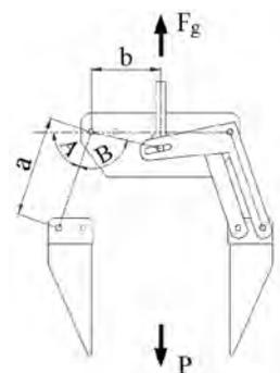
Fig 4. Gripper links and forces
