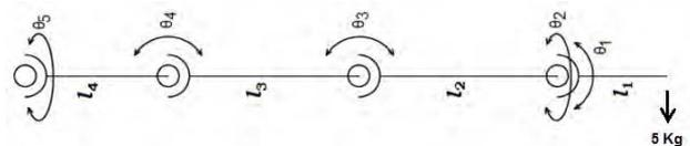
Fig 3. Joints and links of manipulator
