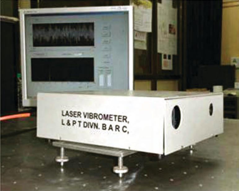
Fig. 1: Photograph of laser Vibrometer sensor with PC interface
