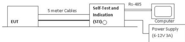
Fig. 2: Test Setup for Seismic Switch.
