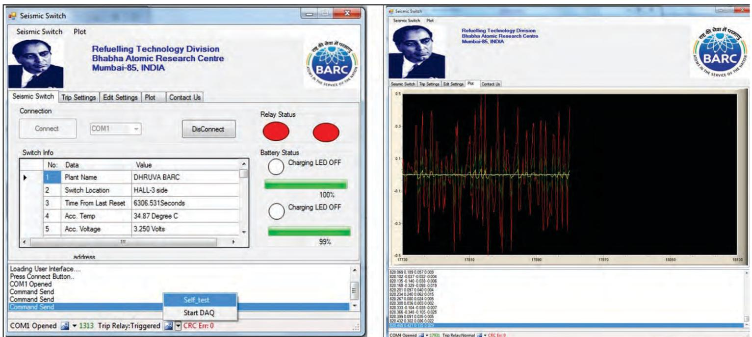
Fig. 3: GUI of the Seismic Switch captured during Seismic qualification testing of the Seismic Switch
