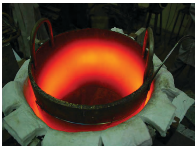
Induction Furnace Heating (~925°C)
