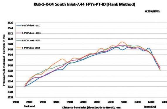
Fig. 5: UT-ID for Channel K-4 KGS-1 (Flank Method)
