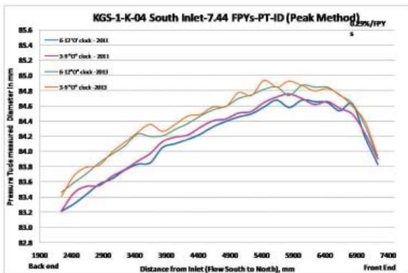
Fig. 6: UT-ID for Channel K-4 KGS-1 (Peak Method)
