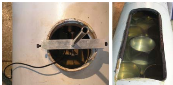
Fig. 3b: Cut-outs for Transducer and FSA Top-heads in 10 m Long Pipe Assembly
