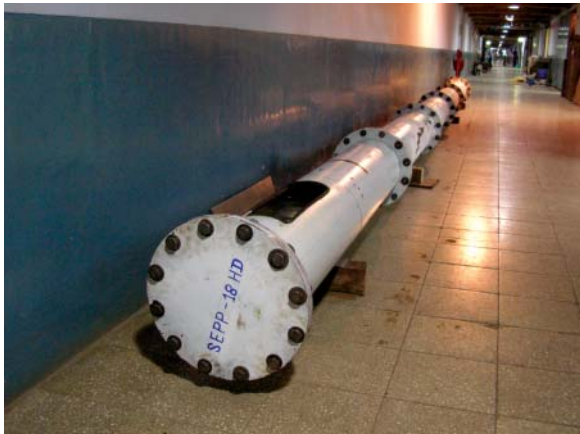
Fig. 3a: 10 m Long Pipe Assembly
