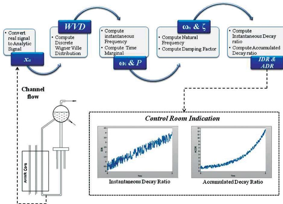
Fig. 5: Time frequency based algorithm for computing decay ratio
