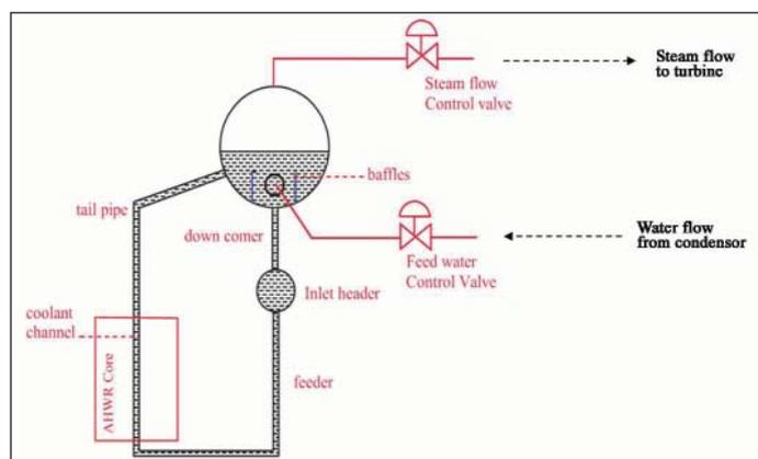
Fig. 1: Main Heat Transport System of AHWR (Schematic)
