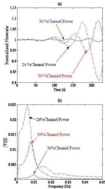
**Fig. 2: (a) Normalised response of channel flowrates at different power levels to a perturbation in power at a fixed inlet subcooling of 24K, (b) Single sided amplitude spectra ( $|Y(f)|$ ) of the normalised channel flowrates**
