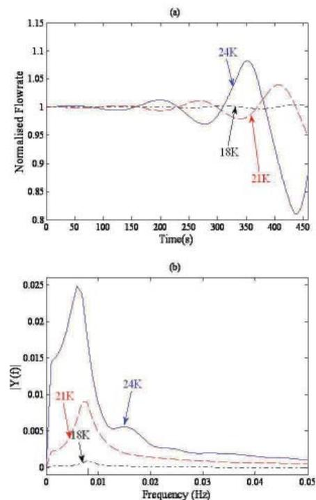
**Fig. 3: (a) Normalised response of channel flowrates at different core inlet subcooling to a perturbation in power around the operating power level of 24% channel power, (b) Single sided amplitude spectra ( $|Y(f)|$ ) of the normalised channel flowrates**
