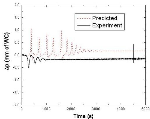
Fig. 7: Comparison of the predicted pressure drop across the heater with the experimentally observed behavior for heater power of 200W
