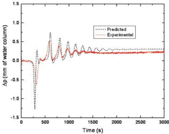
**Fig. 5: Comparison of flow initiation transient predicted by the model developed with experimental behavior for HHVC configuration for a heater power of 257 W.**
