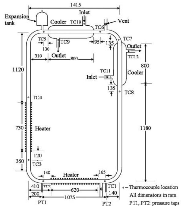
Fig. 2: Schematic of natural circulation loop [8]
