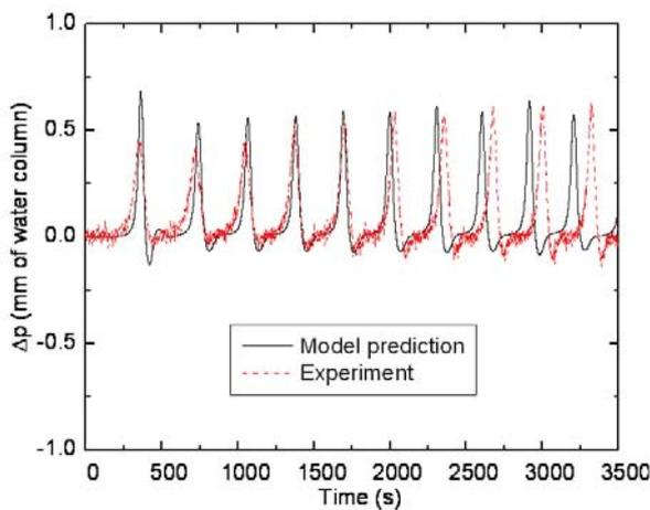
of model predictions with the experimental data for HHHC configuration for a heater power input of 120 W. For this configuration, both loop mass flow rate (indicated by pressure drop across heater) and fluid temperature were found to be oscillating. In fact, for this configuration, stable behaviour was observed only at powers below 55 W.
