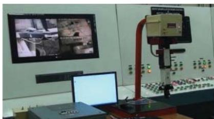
Fig.2: Master Arm of SSM in the Control Room
