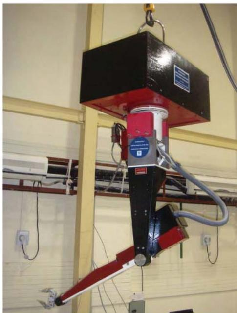
Fig.1: Suspendable Servo Manipulator (SSM)
