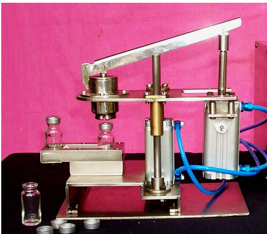
Fig. 2 10ml vial crimping unit installed in ^{131}\text{I} processing plant.
