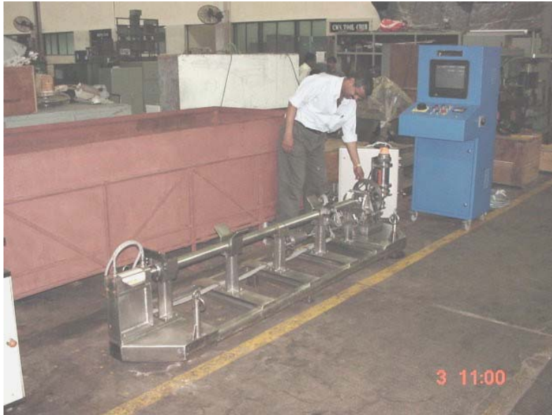
Under water cutting machine
