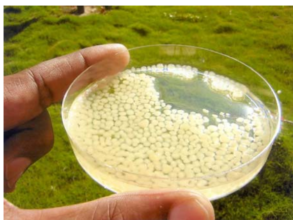
Fig. 1 Aerobic microbial granules cultivated in the laboratory and used for biodegradation studies
