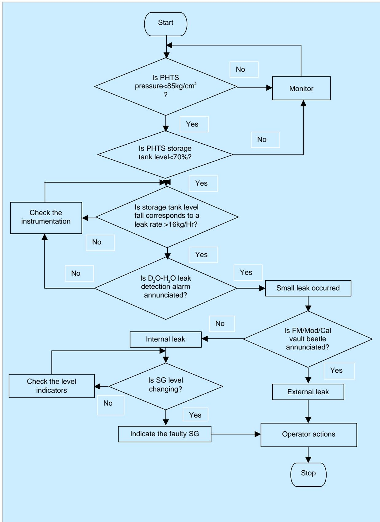
Fig. 2 Event identification flowchart for steam generator tube rupture event
