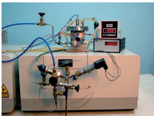
A stainless steel cell for in situ FTIR studies of catalytic processes, under the high-temperature and high-pressure reaction conditions.
