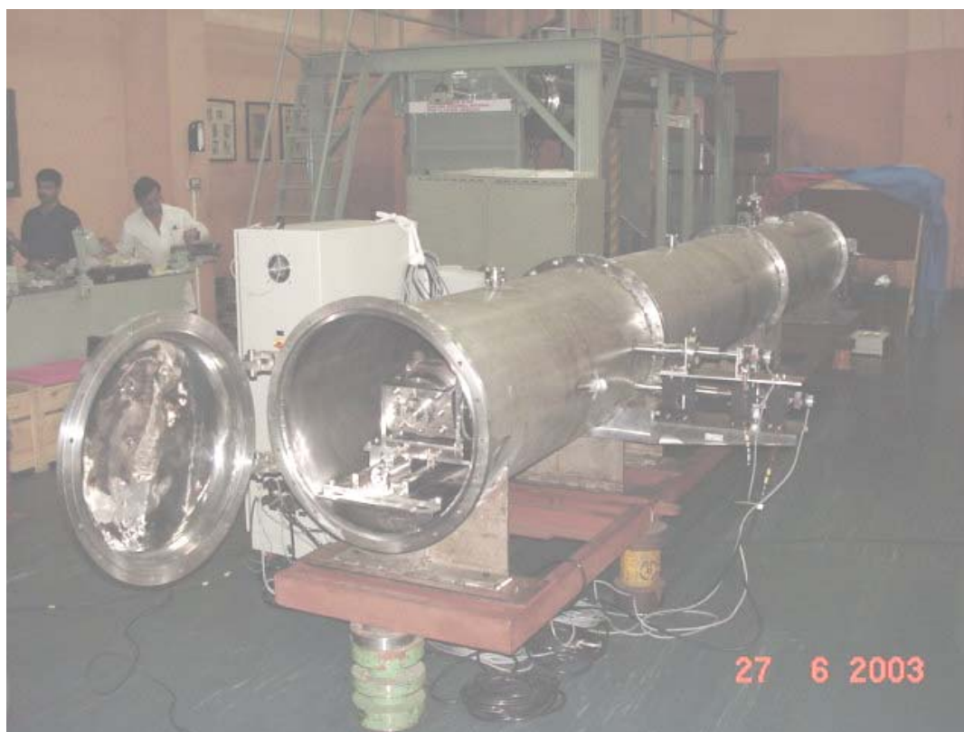
Grating end of spectrometer
