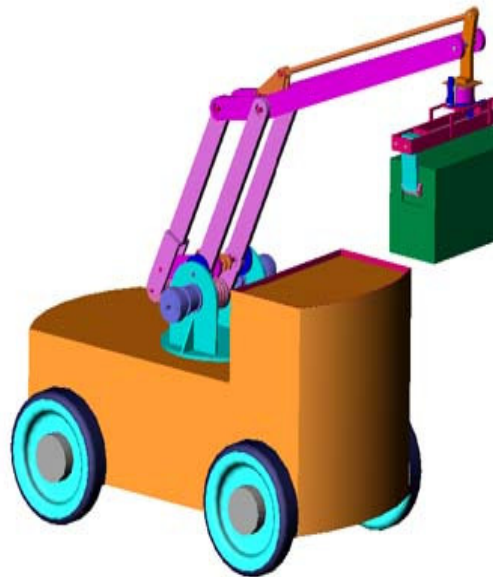
Fig. 6 Mobile robot for removal of boxes containing explosive fuzes.
