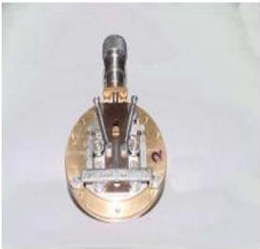
Fig. 4 Internal details of variable opening slit
