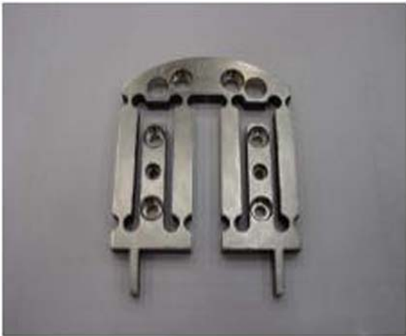
Fig. 2 Four bar mechanism
