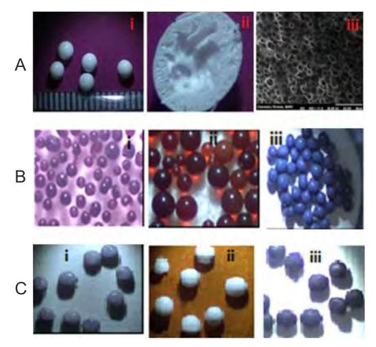
Fig. 1: (A) (i) Optical image of D2EHPA-encapsulated polymeric beads for sorption uranyl ions (ii) crossectional view of the bead (iii) SEM image of the bead (B) Optical images of inorganic sorbent polymer composite beads (i) Resorcinol formaldehyde (RF) bead (patented) (ii) RF-XAD bead (iii) KCoHCF-Gel bead (C) Optical images of inorganic sorbent polysulphone (PS) beads (i) CuHCF-PS composite beads (ii) TiO<sub>2</sub>-PS composite beads (iii) MnO<sub>2</sub>-PS composite beads
