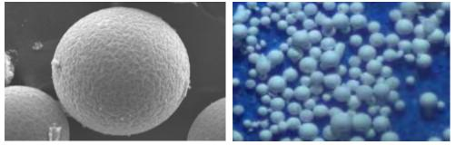
Fig. 2: Polyacrylonitrile based chelating resin for gallium extraction from Bayer's liquor
