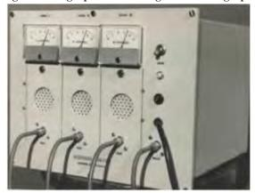
Fig. 3: Three channel hydrogen monitor
