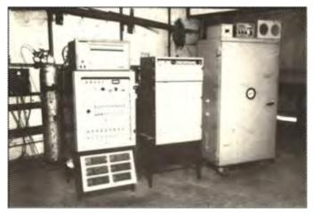
Fig. 4: MAPS cover gas analyzer developed at Chemistry Group, BARC
