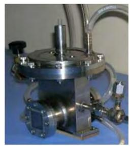
Fig. 3: A SS-cell equipped with Be-windows for *in-situ* EXAFS study of catalytic materials at EXAFS beam line in INDUS-2 at RRCAT, Indore (*developed in collaboration with Applied Spectroscopy Division & CDM*)
