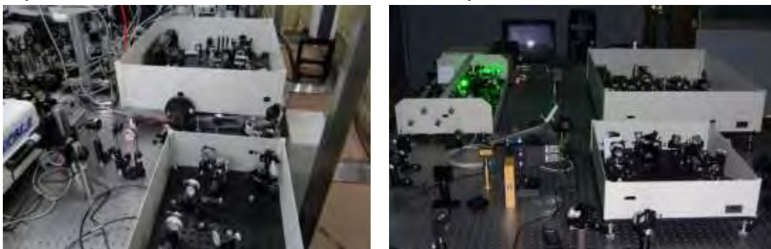
Fig. 2: Two ultrafast facilities to study the condensed phase chemical dynamics: Left- Transient absorption; Right-Fluorescence up-conversion
