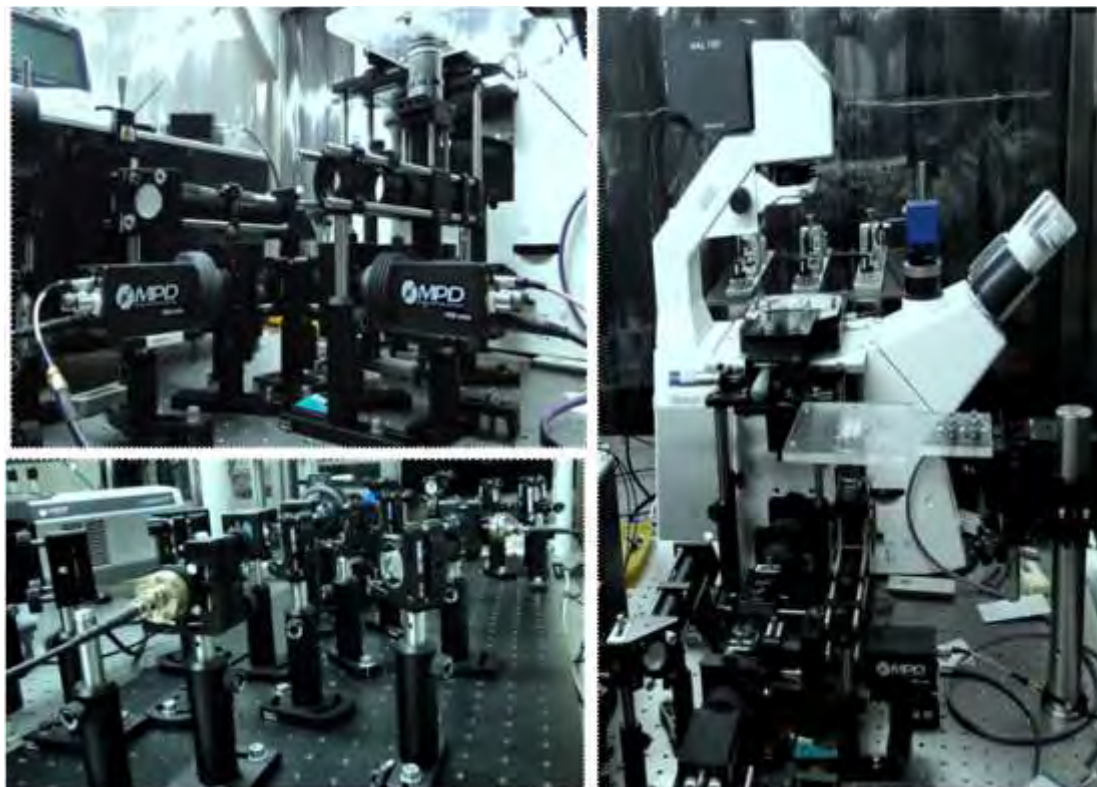
Fig. 5: A home-built single molecule multi-parameter fluorescence spectroscopy setup
