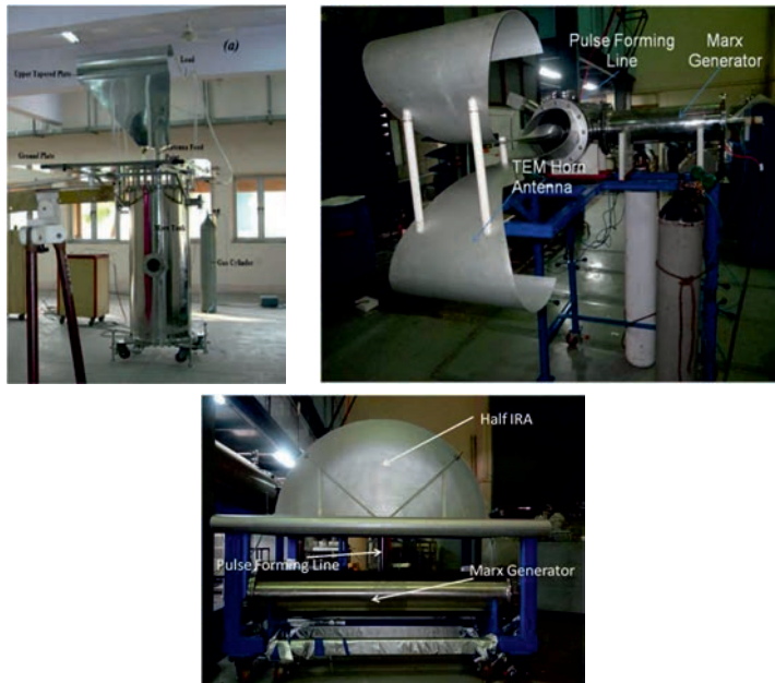
Figure 14.10. Photographs of the UWB system with half TEM horn antenna.
