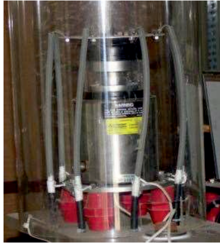
Figure 4.8. Constructional schematic of an elementary ignitron switch and coaxial mounting of NL8900 Ignitron switch having maximum ratings of 35 kV, 300 kA, 250 C.
