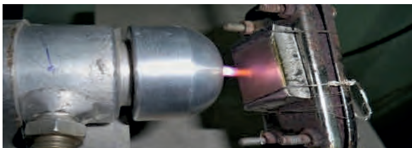
Figure 24.12: Process of plasma nitriding on titanium sample.
