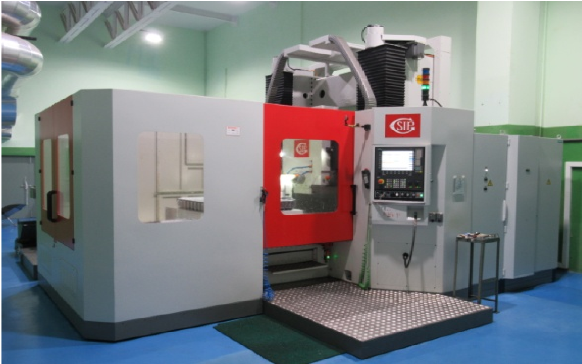
Fig: CNC High Precision Horizontal Boring & Milling Machine (Make: SIP, Switzerland)
