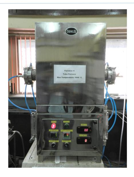
Electrical heating furnace with Ar, N<sub>2</sub>, O<sub>2</sub> Gas flow environment
