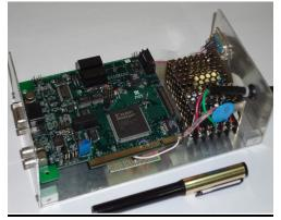
• Eight single ended/ four differential ended 16 bit 100ksps analog inputs with programmable ranges of 0-5V, 0-10V, +5V, +10V.
