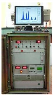
The Quadrupole Mass Spectrometer is a very versatile analytical instrument capable of compositional analysis of gases and volatile liquids. It consists of an Electron Impact ion source, quadrupole mass analyzer and a detector. The QMS is a compact, reliable and low cost analytical tool which has numerous applications in the industry. It can analyse a mass range of 1-300 amu with a resolution of 1 amu, which is adjustable.
