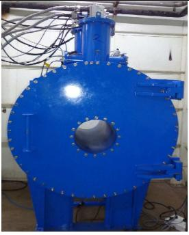
300mm diameter Warm bore superconducting solenoid magnet
