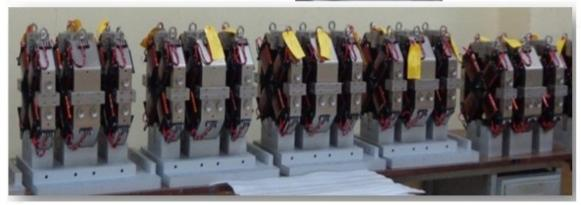
Electromagnetic quadrupoles for MEBT line and quadrupoles and dipole correctors for LBHB 650 MHz section of PIP-II at Fermilab has been designed, developed, characterised and shipped to Fermilab. Quadrupoles are used to provide transverse focusing to the beam. Dipole Correctors are used to provide optical correction and steering to the beam.
