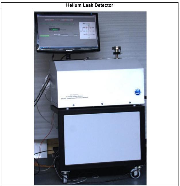
The instrument is primarily useful for the vacuum leak testing of UHV components, chambers, enclosures, vacuum sealings, large experimental facilities etc.
