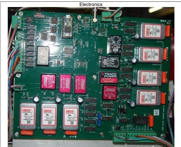
An electronics card developed to control & interlock all electronics parameters of Helium Leak Detector (HeLD) and to monitor the data & present it to the control software (PC) over a serial bus.
