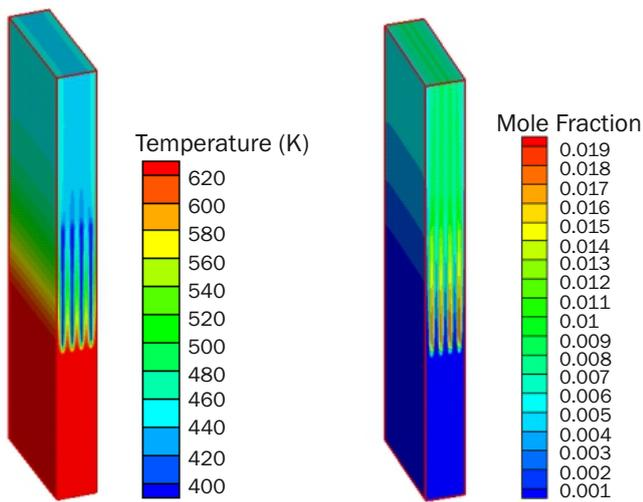
Fig.3: Temperature contours (left) and hydrogen mole fraction contour (right) for simulation performed for REKO facility (Inlet hydrogen mole fraction 2% v/v and inlet temperature 383 K).
