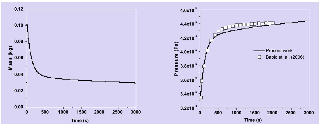
Fig.5: Average hydrogen mass (left) and average pressure (right) in the representative containment.
