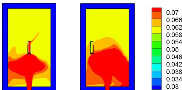
Fig.9: Hydrogen mole fraction contours at 1800 second for case 1 (left) and case 2 (right).
