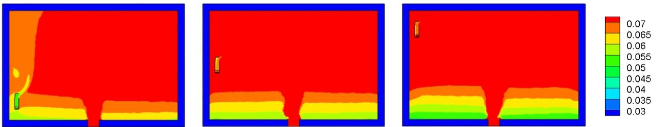
Fig.12: Hydrogen mole fraction contours at 1800 second for case 3-5.
