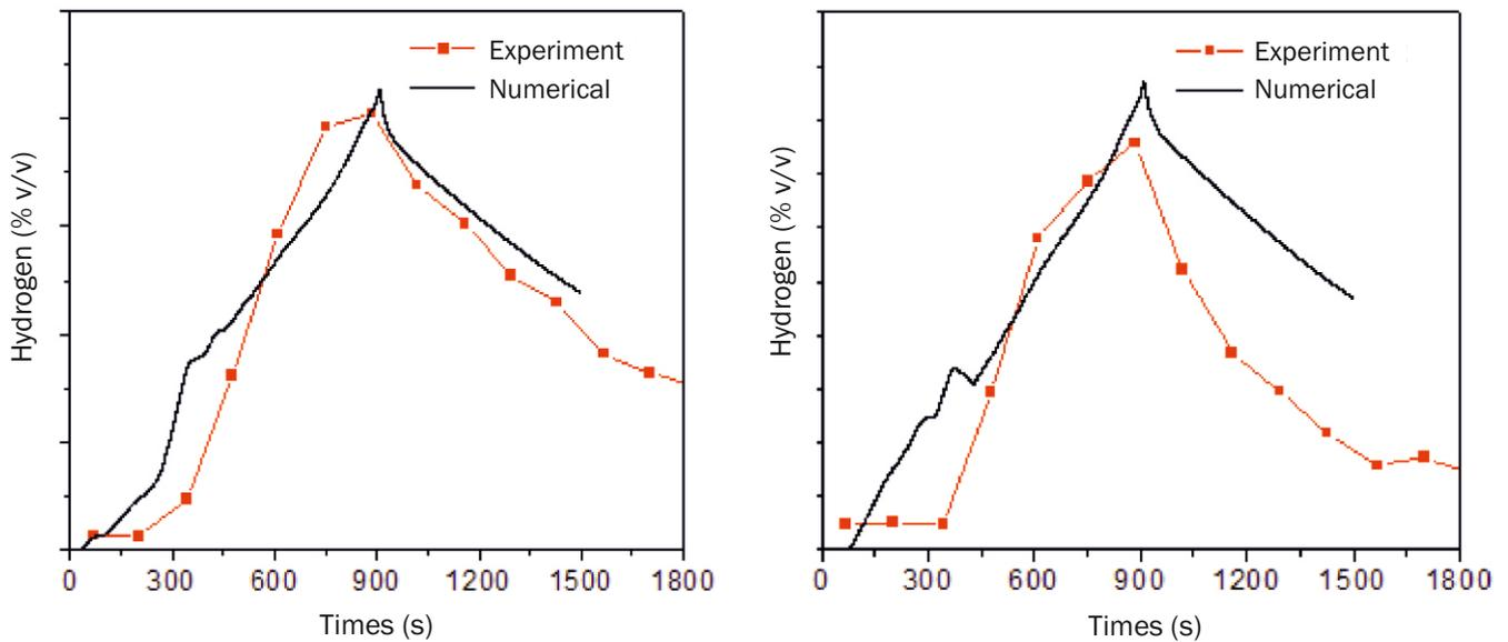
Fig.8: Temporal variation of the hydrogen concentration at PAR inlet (left) and outlet (right).
