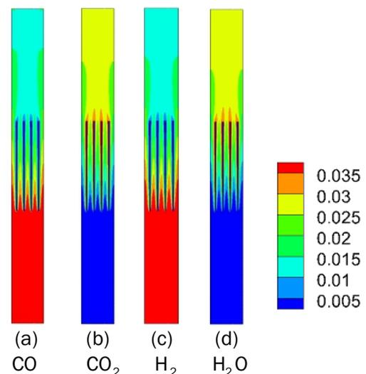
Fig.15: Mole fraction contours of various species ( $CO= 4\%$  (v/v) &  $H_2=4\%$  (v/v) at inlet).
