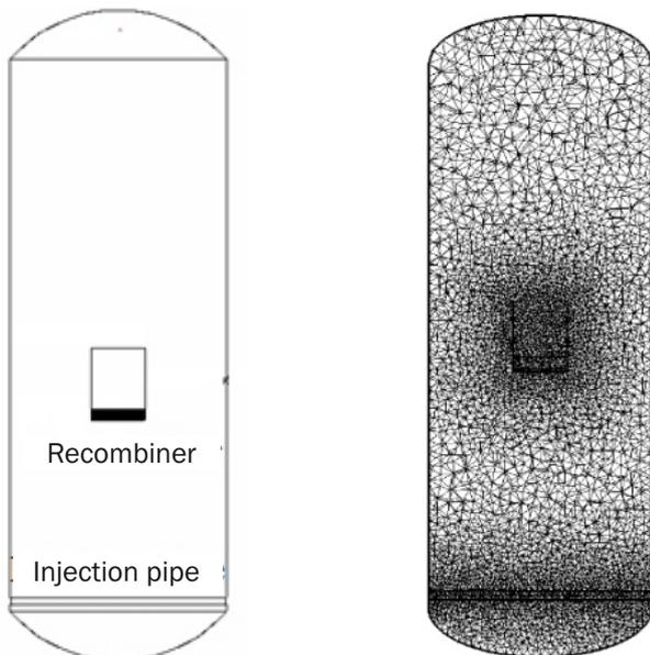
Fig.7: HRTF geometry (left) and mesh (right), PAR at center configuration.
