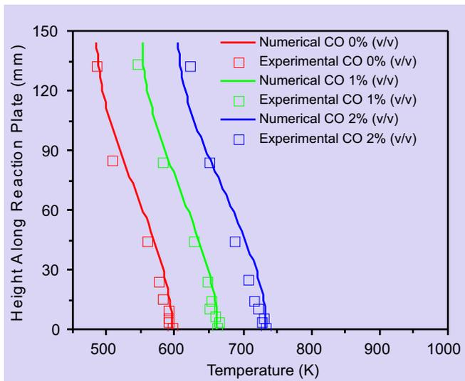
Fig.14: Comparison of computed plate temperatures with experiments for different CO concentration at inlet ( $H_2$  2% (v/v) at inlet).
