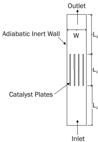
Fig.1: Simplified geometry of Plate Type PAR for 3D CFD computation.
