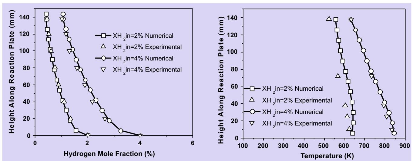
Fig.2: Steady state average hydrogen mole fraction in the recombiner section of REKO facility (left), catalyst surface temperature along the catalytic plate (right), (Inlet hydrogen mole fraction 2% & 4% and inlet temperature 343 K).
