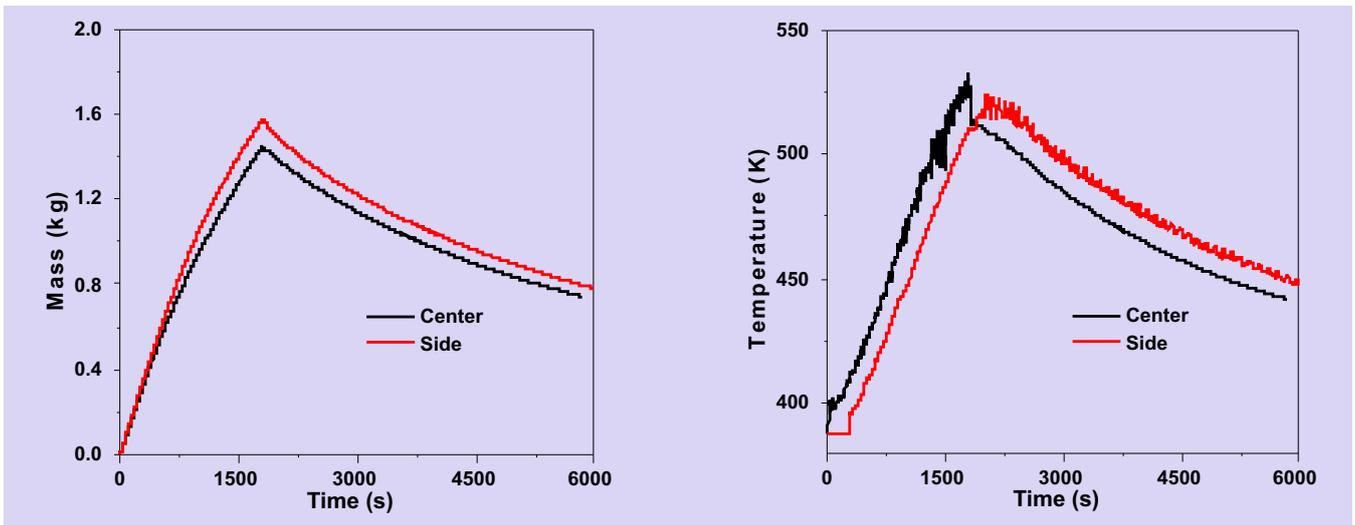
Fig.11: Temporal variation of total hydrogen mass (left) and PAR outlet temperature (right) in enclosure for case 1-2.
