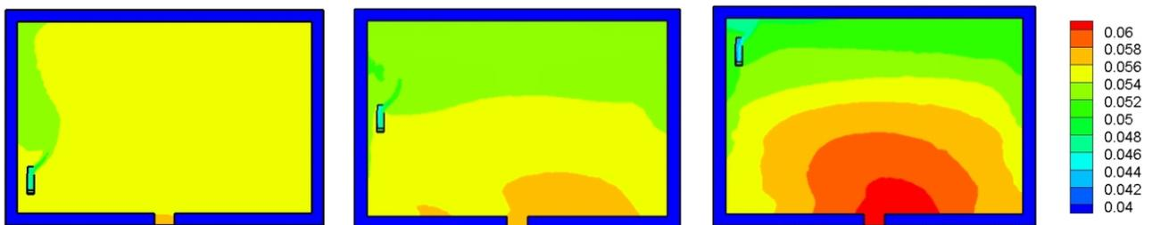
Fig.13: Hydrogen mole fraction contours at 18000 second for case 3-5.
