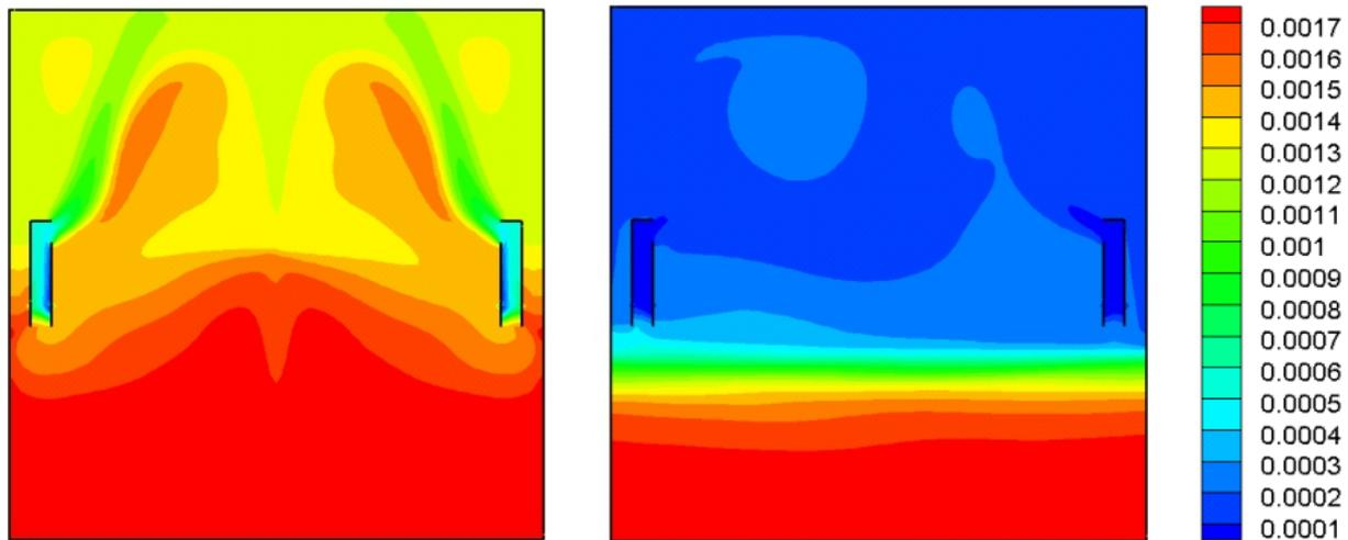
Fig.6: Hydrogen mass fraction at 20 s (left) and 300 s (right).
