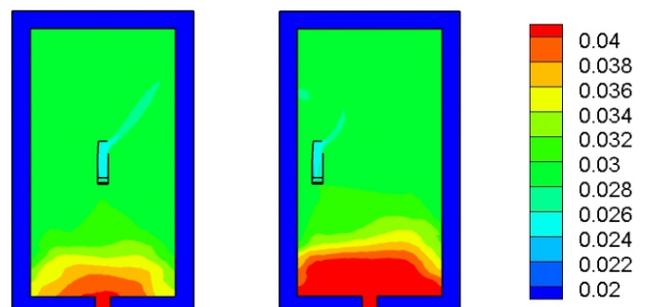
Fig.10: Hydrogen mole fraction contours at 6000 second for case 1 (left) and case 2 (right).
