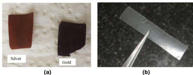
Fig.3: (a) Photograph showing pieces of silver nanoparticles embedded alginate film (left) and gold nanoparticles embedded alginate film (right) and (b) Alginate film.
