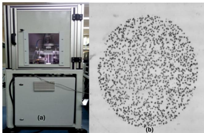
Fig.5: (a) Automated imaging system (b) Tracks in CR-39.
