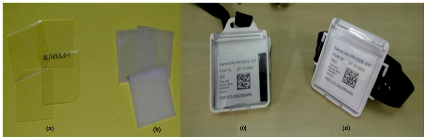
Fig.4: Neutron Badge components (a) CR-3 foils (b) Polyethylene radiator (c) Chest badge and (d)Wrist badge.
