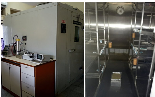
Fig.5: Outside and inside view of the calibration chamber.
