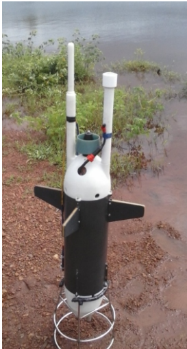
Fig.1: Autonomous Vertical Profiler (front side view).
