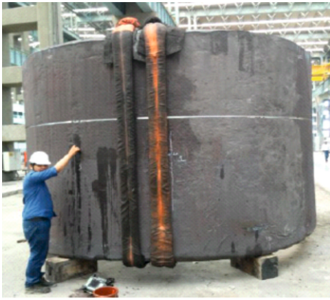
340 mm thick Shell Forging for Nozzle Area of RPV-OD4900 x ID4220 x 2000L
