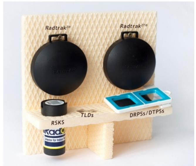
Fig.13: DRPS/DTPS in RaThoGamma kit of environmental radioactivity measurement in Romania [11].
