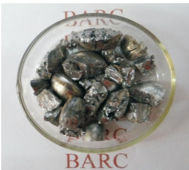
Fig.5: Crushed alloy button before loading in the reactor
