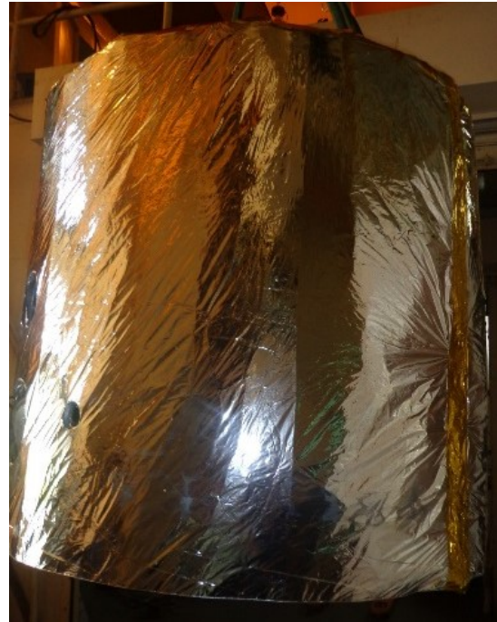
Fig:13 MLI blanket wrapped over thermal shield
