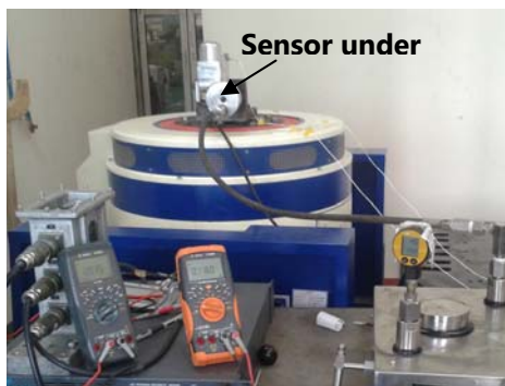
Fig.5: Vibration test of Absolute Pressure Sensor
