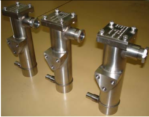
Fig.3: LOCA qualified Absolute Pressure Sensor mark-II
