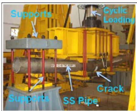
Fig. 1: Cyclic Tearing Tests- Four Point Bend Loading Setup
