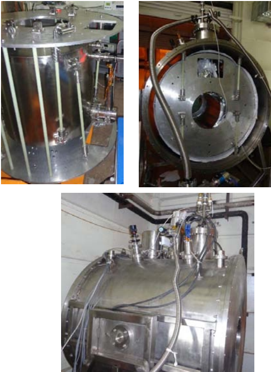
Fig:15 Assembly of SC magnet
