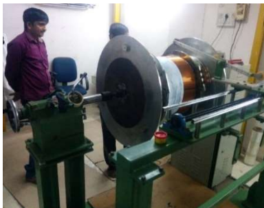
Fig. 4: SPM developed to carry out winding
