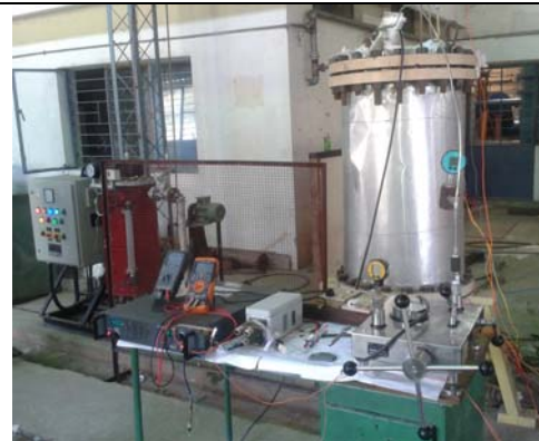
Fig.4: Absolute Pressure Sensor placed inside the environmental chamber for qualification tests
