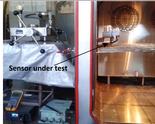
Fig.4: Absolute Pressure Sensor placed inside the environmental chamber for qualification tests
