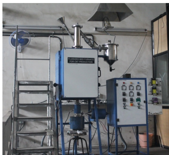
Fig. 1: Fluidized bed furnace for CNT production
