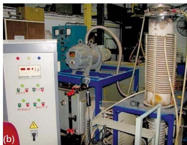
Fig.1: a) Schematic and b) actual photograph of a vacuum induction furnace used for synthesis of  $(Ti,Cr)B_2$  and  $MoSi_2$
