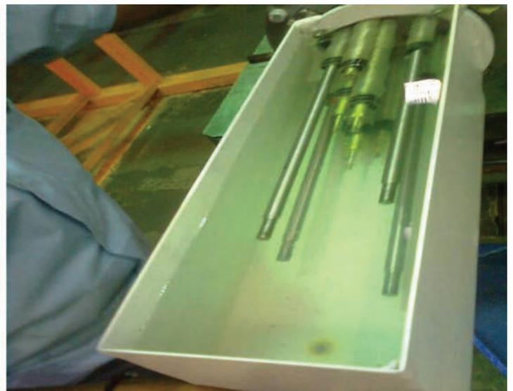
**Fig. 3: Leak testing of Individual Component**
