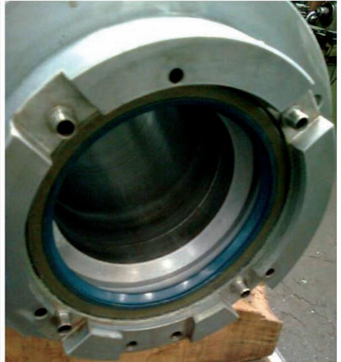
**Fig. 2: Installation of Dynamic seal**
