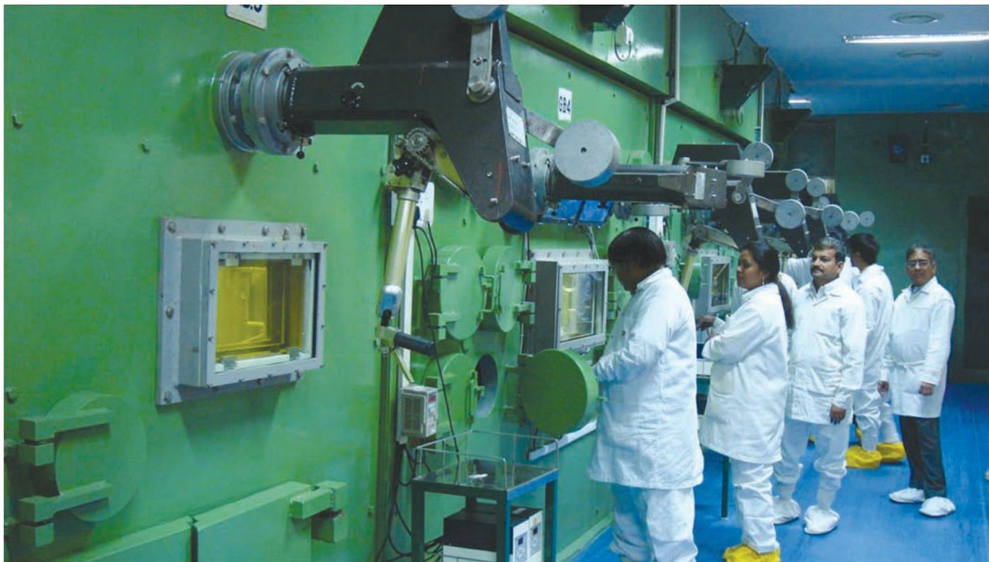
**Fig. 8: Leak Tight Articulated Manipulators in Operation at PRTRF Lab**
