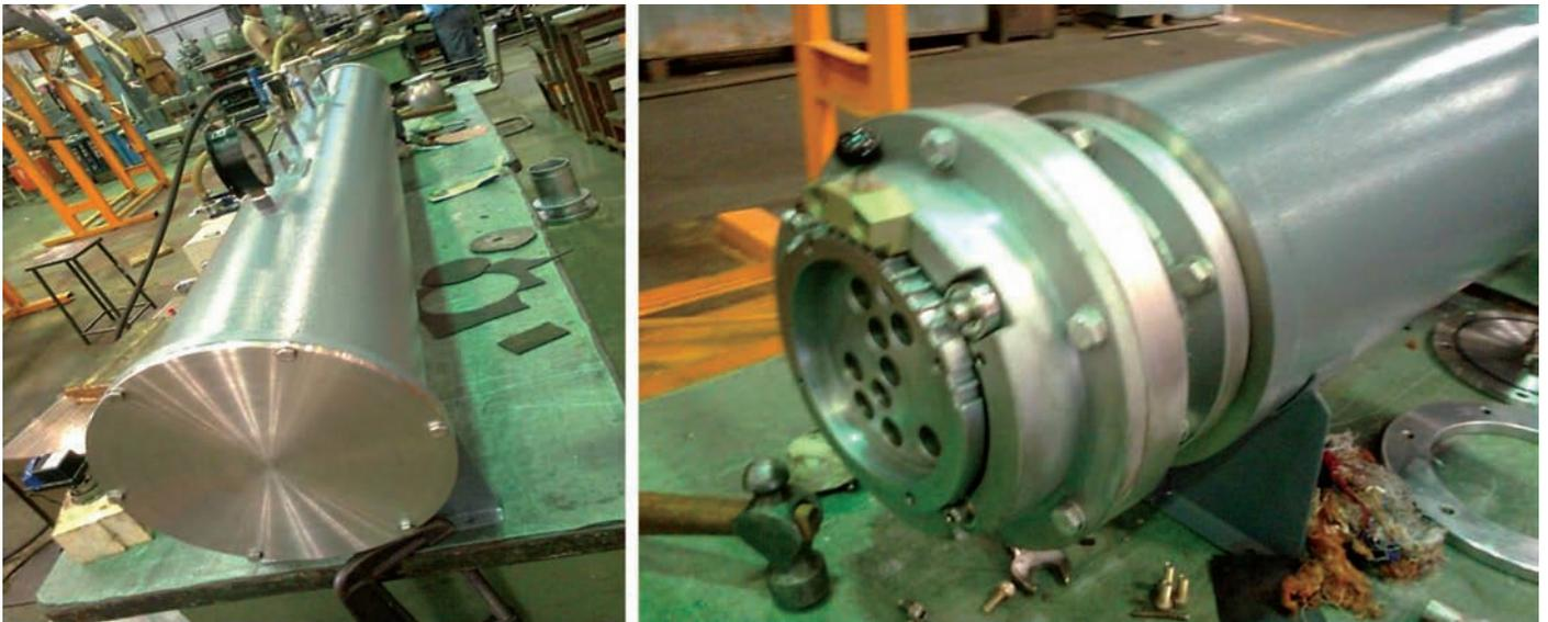
Fig. 4: Actual set up for Leak testing
