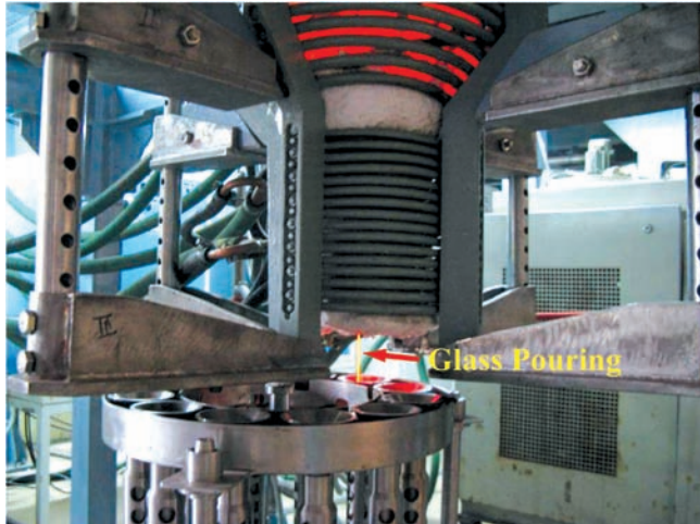
Fig. 6: Pouring of vitrified Product in Pencil
