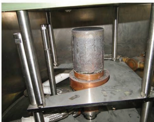
Stainless steel ingot after in-situ casting
